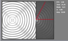
Figure 4. Diffraction effects studied by varying width of the slit. Slit width = 4 units. Angle of diffraction = 63 deg.
