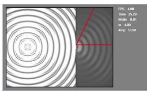
Figure 6. Diffraction effects studied by varying frequency (wavelength). Frequency = 4 Hz. Angle of diffraction = 64 deg.
