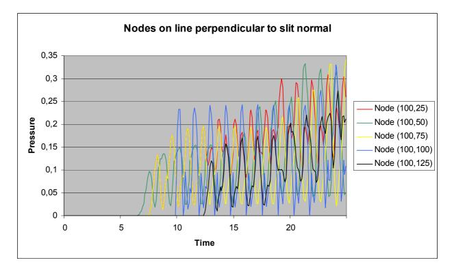
*Figure 8. Pressure at nodes on a line perpendicular to the normal vector of the opening. Five nodes ploted in the same diagram.*
