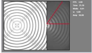
Figure 5. Diffraction effects studied by varying width of the slit. Slit width = 8 units. Angle of diffraction = 55 deg.
