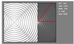
Figure 7. Diffraction effects studied by varying frequency (wavelength). Frequency = 6 Hz. Angle of diffraction = 53 deg.
